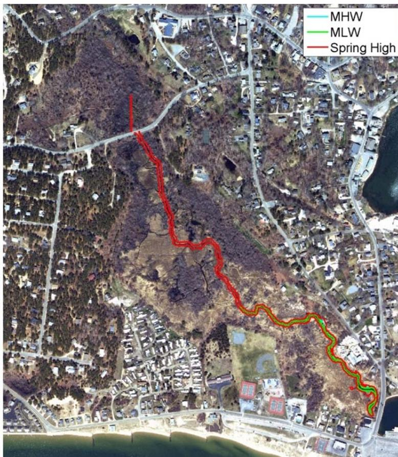
Figure 22. Mayo Creek Basin with contours of MHW, MLW, and Spring High tide under existing conditions (does not consider rainfall).
