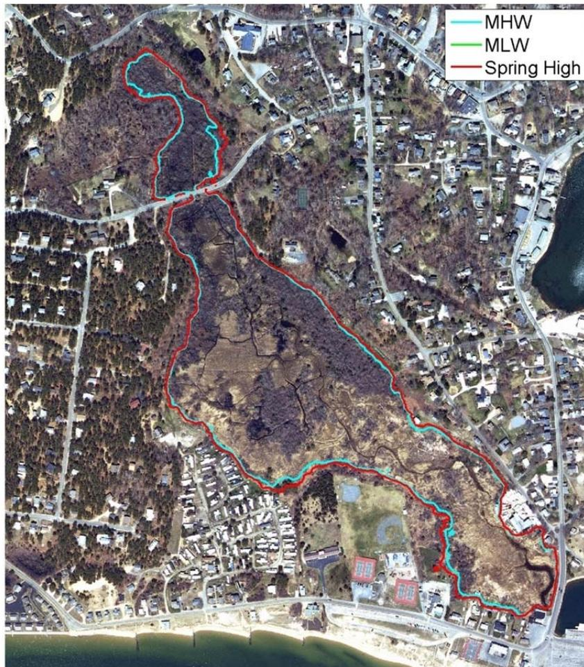
**Figure 34.** Mayo Creek Basin with contours of MHW, MLW, and Spring High tide, forty inch pipe alternative.
