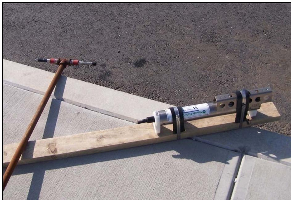
**Figure 5. In-Situ aqua TROLL 200 and Seabird Electronics SBE37 Microcat prior to deployment.**
